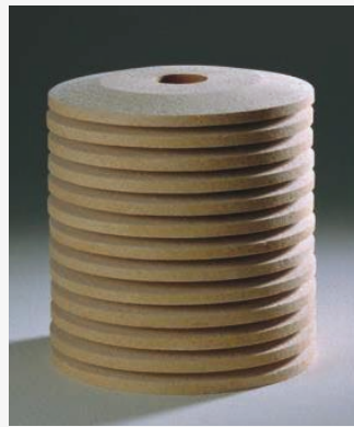
Microfilter cartridge TFP 1000 heat treated Dirt absorption: 2,000 g Filter fineness 3 \mu m absolute including set of seals
